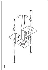
Disconnect the power by turning off the circuit breaker, or by removing the fuse in the fuse box before assembling and mounting the canopy. Fix the mounting plate to the ceiling with the dowels and screws.
