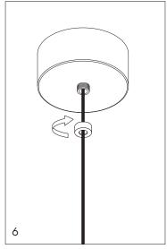
Fix the ceiling rose cover with the fixing
