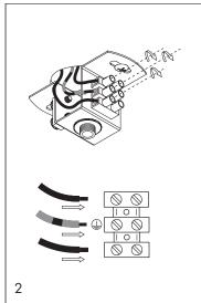
Connect the cable to the terminal block.
