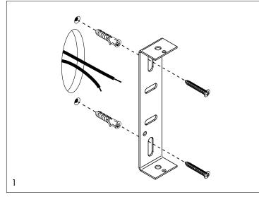
Disconnect the power by turning off the circuit breaker, or by removing the fuse in the fuse box before assembling and mounting the canopy. Fix the mounting plate to the ceiling with dowels and screws.
