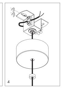
Fix the lamp cable with the fixing bracket on the side to double secure.
