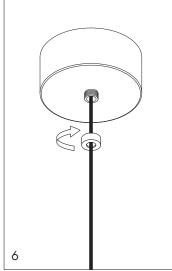
Fix the ceiling rose cover with the fixing nut.
