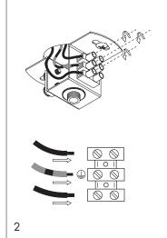
Connect the cable to the terminal block.
