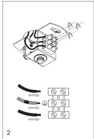
Connect the cable to the terminal block.
