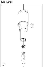
Lift the brass and glass parts. Insert the G9 bulb.
