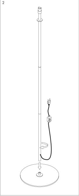
Screw the metal base to the tubes. Make sure that you screw the
