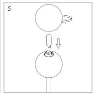
Insert the G9 bulb and screw the glass sphere into the socket. Take care to screw the glass sphere gently.
