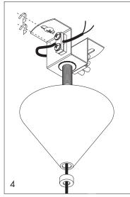
Fix the lamp cable with the fixing bracket on the side to double secure.
