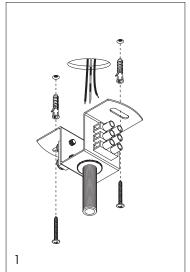
Disconnect the power by turning off the circuit breaker, or by removing the fuse in the fuse box before assembling and mounting the canopy. Fix the mounting plate to the ceiling with the dowels and screws.
