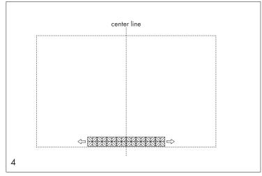
Start to glue the tiles at the bottom and in the middle of the marked area.
