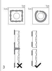
The glue can be applied in a circle or in a square shape around the hole of the tile. The distance between the adhesive and the outer edge should be bigger than 1cm otherwise the adhesive may leak out.
