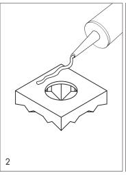
You can use any adhesive or silicone suitable for the installation of tiles. Please take note, silicon variates depending on the surface to be glued. We suggest to use "No More Nails®". Apply the adhesive on the back of the tile.
