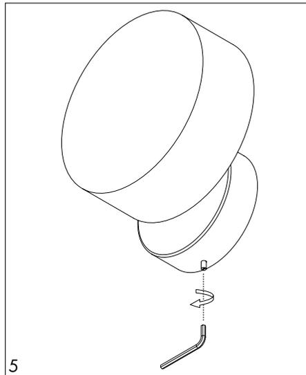
5 Fix the lamp with the allen screw into the mounting plate.
