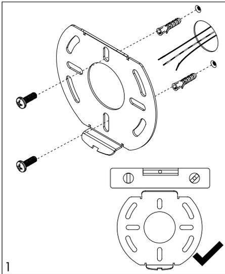
1 Fix the mounting plate to the wall with dowels and screws.
