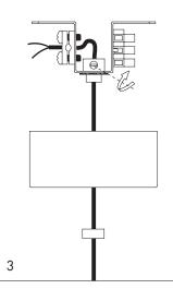
Fix the lamp cable with the fixing screw on the ceiling box. Take care to screw the screw gently but firmly
