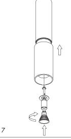
Lift the brass and wood part. Insert the GU10 bulb. Warning: Use only LED
