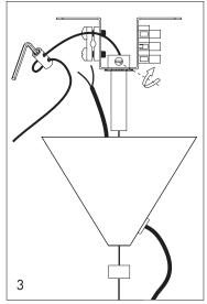
Adjust the height of the lamp with the metal cable and fix the desired height with the on the side to double secure. hex key. Cut the excess of the metal cable if necessary.
