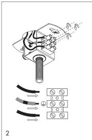
Connect the cable to the terminal block.
