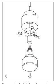
Unscrew the plastic bolts and remove the glass. Exchange the Gu10 bulb **Warning:**Use only LED
