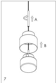
Unscrew the part A. Lift part A and B.
