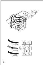
Connect the cable to the terminal block.
