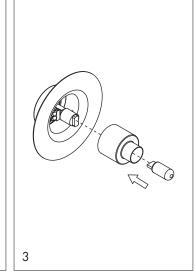
Cover the technic with the metal cover and insert the G9 bulb. **Warning:** Use only LED
