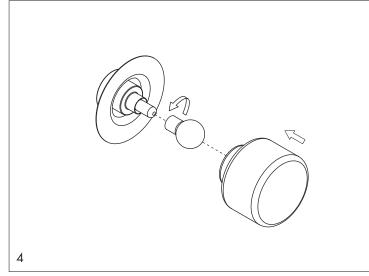
Fix the metal cover with the glass sphere. Take care to screw the glass sphere gently.
