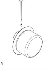
Fix the recycled handblown glass with the PVC grub screws
