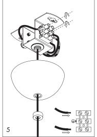
Connect the cable of the lamp to the terminal block.
