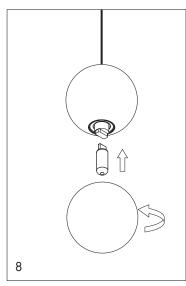
Insert the G9 bulb and screw in the metal tube. **Warning:** Use only LED
