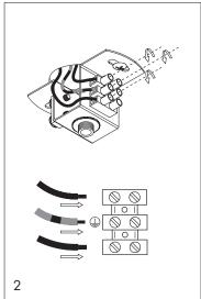
Connect the cable to the terminal block.
