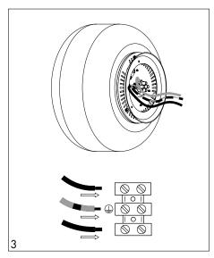
Connect to electricity using the terminal block.
