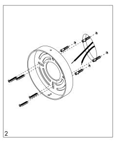
Fix the mounting plate to the wall with dowels and
