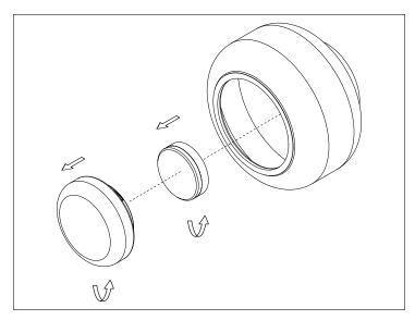
**Bulb change:** Spin off the inside opal glas, the spin off the Gx53 Bulb.
