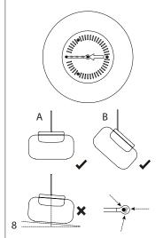
Gently pull the cable through the rail to fix position and place into the opposite edge.
