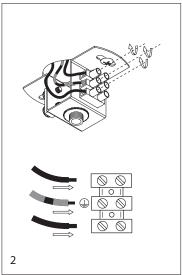
Connect the cable to the terminal block.
