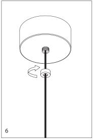
Fix the ceiling rose cover with the fixing nut.
